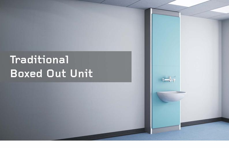
Our original healthcare boxed out unit features large access panels and has aluminium corner extrusions providing extra protection. The unit can be quickly and simply fitted to the wall using brackets and secured with tie back rods. Panels are available hinged and lockable and allow wide access points to services behind.
