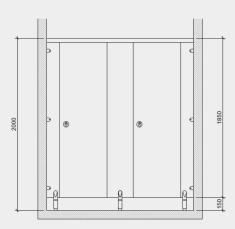
TYPIEAL CUBICLE FRONT ELEVATIONS
